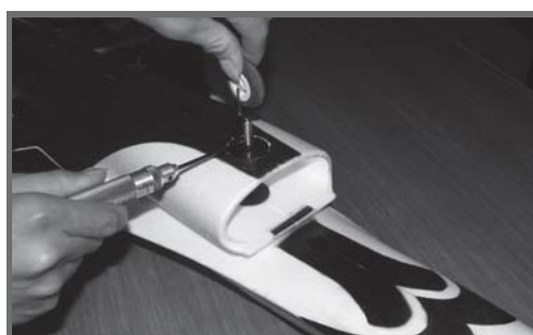
3.4 Slide the nose gear into the slot from the bottom of the fuselage. Use a hexagon screwdriver to tighten the screw.
