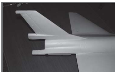
2.2 Fit the vertical stabilizer to the fuselage and remove excess glue.
