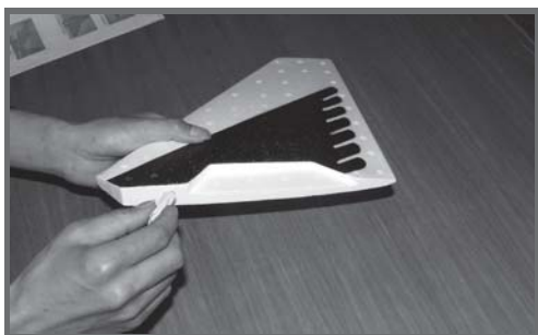
1.1 Apply the foam glue on the joiner of the left and right wing respectively.
