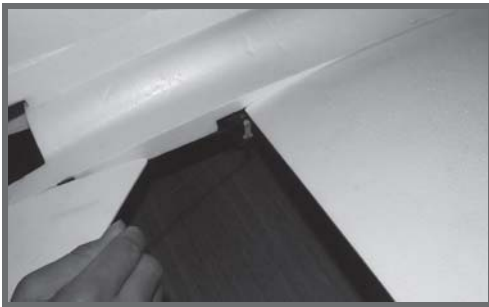
5.1 Insert Z-bend of elevator pushrod into the hole of the servo arm.
