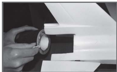
6.1 Apply foam glue to the exhaust nozzle and insert into the fuselage.
