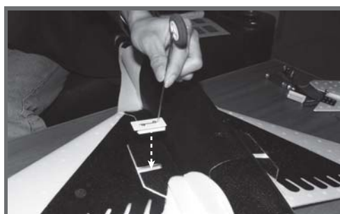
3.2 Push the left landing gear in the position and allow the glue to dry.
