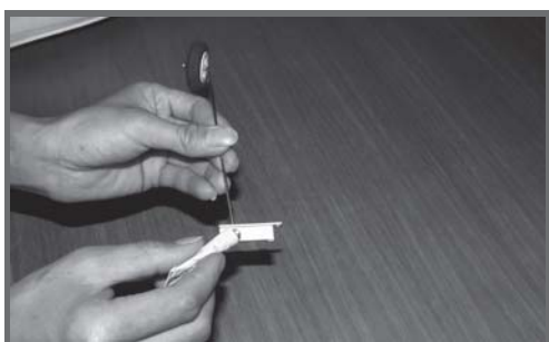
3.1 Apply the foam glue on the joiner of the landing gear.
