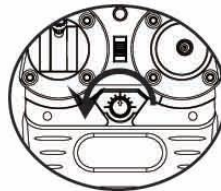
Counterclockwise rotation vernier adjustment knob
