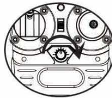
Clockwise rotation vernier adjustment knob
