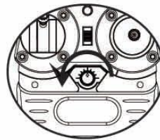
Counterclockwise rotation vernier adjustment knob
